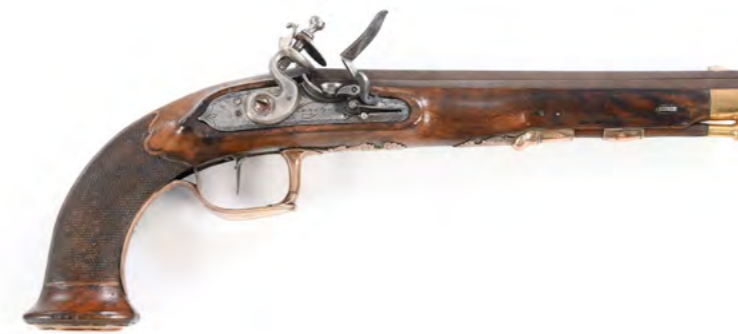
121 Rifled flintlock dueling pistol signed "Manufacture". Rifled octagonal Damascus barrel with rear and front sight. French (Boutet) style stock with red copper engraved furniture. Flat lock with a roller between frizzen and spring. Mounted on the spring. Ca. 1800. Length 36.5 cm. Barrel length 21 cm. Caliber bore 12 mm (ca. kal 40).
