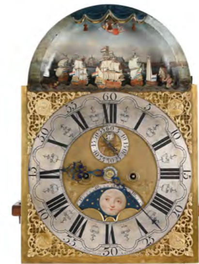
6 A longcase clock by Jan Christ Sauer, with ship mechanism of a fleet on the IJ estuary in front of Amsterdam, a mermaid with a mirror, a merman with a horn and Mercury, the god of trade and industry, floating under a cloth. Oak case, veneered with burr walnut and marquetry, eight-day movement with anchor escapement, subsidiary seconds, moon phase and alarm on a bell. Amsterdam, around 1780. H. 290 cm.
